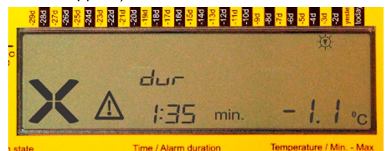
Figure 7 Visualizing the history of a Fridge-tag with preset alarm level violations – Second display
